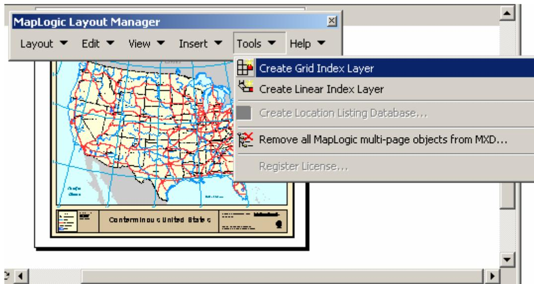
This will display the Grid Index Wizard dialog. In the dialog we must set the limits of where we would like to create a grid for (the grid extent), the size of each grid rectangle, and the file that we would like to store the results in.
